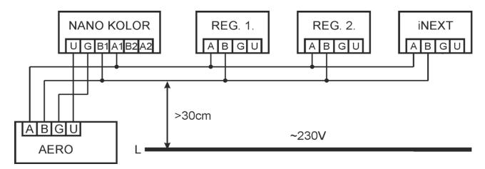
**NOTE:** In order to ensure smooth data transmission it is necessary to install a ferrite filter on the power and communication wires between the AERO module and the NANO COLOR thermostat. When leading the conductors through the filter loop them around the ring as shown in the photo at the side.
