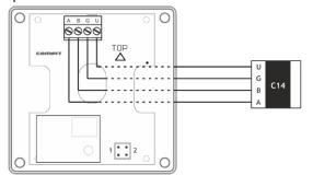
The setting of jumper links No. 1 and No. 2 defines the VSHC sensor address in C14 network. The sensors can have numbers from 6 to 9.
