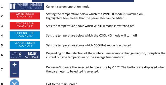
**NOTE:** The difference between the temperatures WINTER START and WINTER STOP, WINTER STOP and COOLING STOP, COOLING STOP and COOL START must be at least 1°C. When increasing the temperature, this difference automatically transfers to the other settings.
