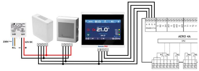
Note! Up to 4 VSHC or VSHW sensors and one VACS-1 sensor can be connected to the device.
