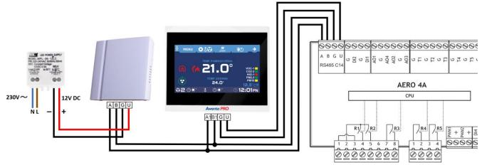
Note! Only one VACS-1 or VSPM sensor can be connected to the device.
